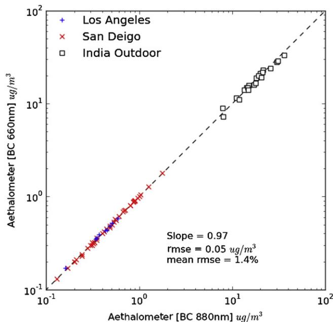
Fig. 3. Compares the Aethalometer [BC] at 880 nm where brown carbon absorption is negligible, with that at 660 nm. The two [BC] values agree within 5%.
