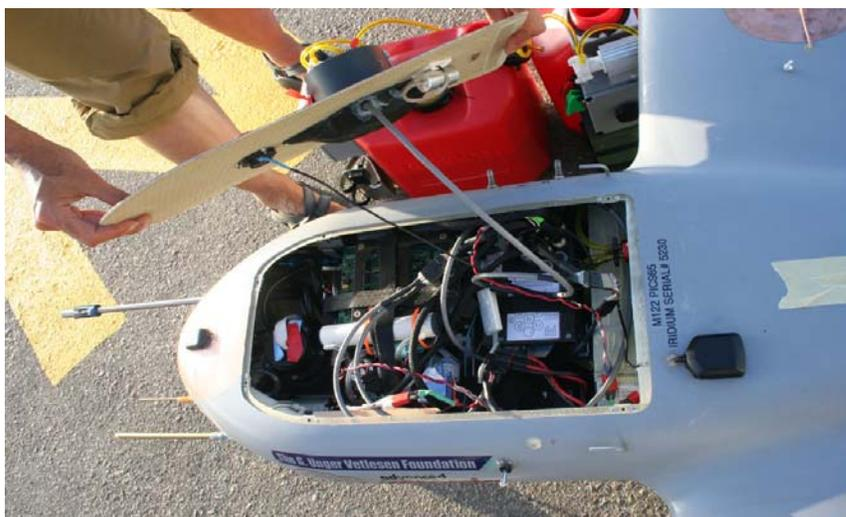
**Figure 13:** Payload bay for instrumented aerosol-radiometric AUAV.
