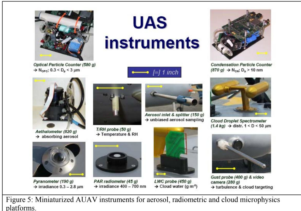
**Condensation Particle Counter (CPC):** The CPC measures total aerosol concentrations between 0 and  $10^5 \text{ cm}^{-3}$  in the diameter range ( $0.01 \mu\text{m} < D < 1.0 \mu\text{m}$ ). The CPC serves as a reference for comparison with other aerosol measurements, and as an indicator for clean versus polluted regimes. The Model 3007 is TSI's smallest CPC and has been integrated into the fuselage of the AUAV.
